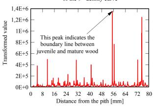
Figure  $4 - 2^{nd}$  Fourier spectrum of density distribution of sample nr. 9.
